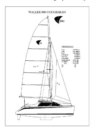
replaced on a regular basis for safety. Pounding in heavy weather is reduced by keeping the bridge deck as high as possible above the water, and by the use of chamfer panels between the hulls and bridge deck, which pick up extra buoyancy as waves travel between the hulls. It must be noted that small cats of this configuration have safely completed major ocean voyages, including circumnavigations.
