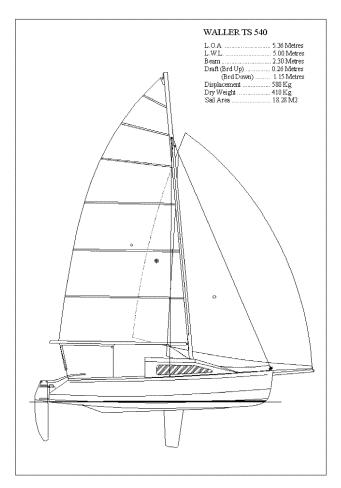
same excellent sailing and handling characteristics, but which could be built from sheet ply wood. Like the TS 5.4, the Waller TS 540 is designed for two people, and is ideal for a couple, or parent and older child. (Of course, more can be carried for day sailing.) The small cabin contains minimal overnight 'camping' accommodation, with two bunks in the traditional 'V' berth configuration. Removable panels allow these berths to convert to a comfortable sitting area for two people.
