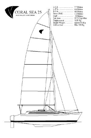
The Coral Sea 25 is the smallest in the Coral Cat range, and is a simple truncated 'V' hull cat designed for the builder who wants the most boat for the least bucks. The vessel has separate hulls joined by solidly mounted cross beams, and is demountable for trailing if desired. The truncated 'V' hull is exceptionally simple to construct, being as easy as the straight 'V' but with better sailing characteristics such as less wetted surface, better tacking etc.
