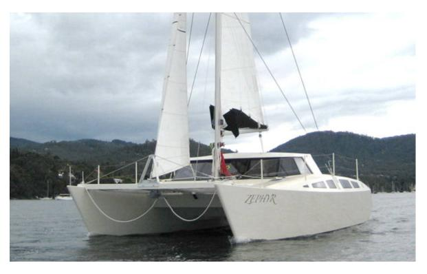
The CORAL COVE 31 CATAMARAN has been designed to specifically to fill the role of an open water capable small family cruiser for coastal cruising and short term on board living, but at a reasonable cost. Hull shape, rig and accommodation layout have been designed with this aim. In general, the boat is optimized towards a cruising family, with more emphasis on livability than in the maximum number of births.
