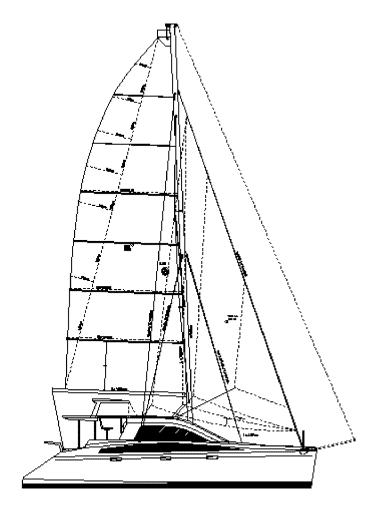
battened main and 7/8th rig which time has shown to be the most efficient rig for this type of vessel.
