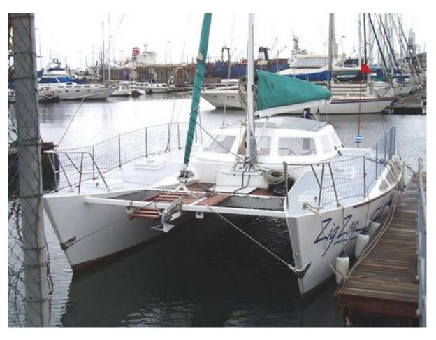
The Coral Sea 35 is designed specifically for the builder who wants maximum boat for minimum cost and building time. To this end the vessel features a simple truncated 'V' hull shape, and separate hulls connected by strongly mounted cross beams. These beams are <u>not</u> flexibly mounted. The truncated 'V' hull is exceptionally simple to construct, being as easy as the straight 'V' but with better sailing characteristics such as less wetted surface, better tacking etc.
