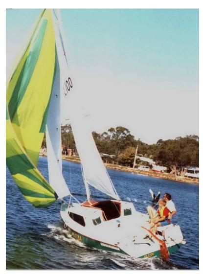
minimum utilising basic 'off the shelf' items. Spars can be constructed at home from stock alloy sections. Plans allow for an asymmetrical kite to be flown from a bow pole, or the option of a normal spinnaker set from a pole on the mast.
