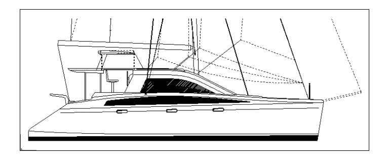
The WALLER 1200 is a full bridge deck cat built in cedar strip/glass composite and plywood. She is an (almost) all plywood version of our 1160 catamaran, with only minor styling changes to accommodate the extensive use of plywood (the 1160 is all strip plank / composite construction).
