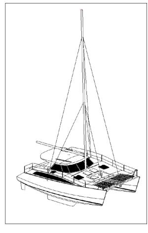
The WALLER 1100 is a full bridge deck cat built entirely from marine plywood, to produce a sound and comfortable ocean cruising vessel at a lower cost than is typical of cats built in most other materials. She is a medium displacement cat intended to be easy and inexpensive to build, and suitable for living aboard and ocean voyages. Because she is intended for extensive cruising, she has been designed with slightly wider hulls for load carrying ability and internal space.
