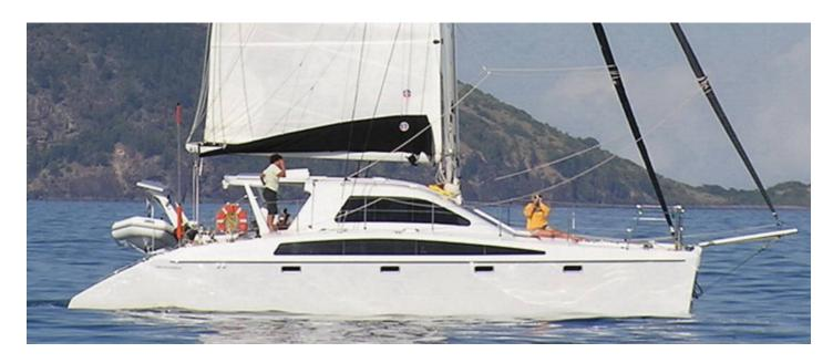
The WALLER 1160 is a full bridge deck cat built in cedar strip/glass composite, to produce a sound and comfortable ocean cruising yacht. Paulownia or Duracore could be used as alternatives. Bulkheads and partitions are in plywood, with interior joinery in honeycomb composite panels.
